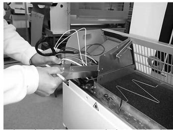
The pc board SIReB1 must be loosened and pulled out a bit to be able to remove the water coil.
