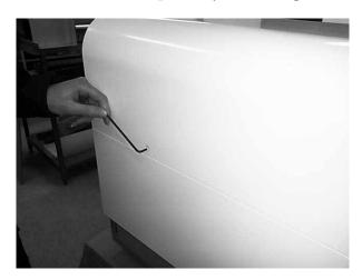
The front shall be locked in open position using the front hatch hook. The hook should afterwords be removed from the old coil to be refitted on the new coil.
