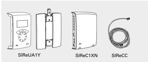
Manual or automatic control of fan speed and temperature with an integrated thermostat. Possibility of selecting whether the fan should be switched off or not at set room temperature, depending whether sound comfort or circulation of room air is prioritised. Possibility to change preset values for each fan step (SWH EC).
