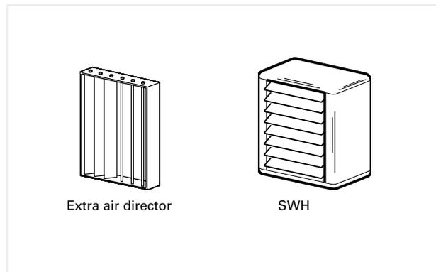
The air throw data is valid at fan position 4 and room temperature +18 °C. The air throw is defined as the distance in a straight angle from the fan heater to the point where the average air speed has dropped to 0,5 m/s.
