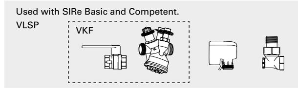
VLSP, pressure independent valve system on/off
