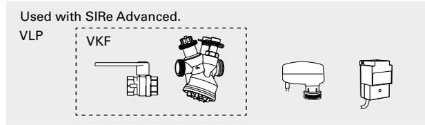
VLP, pressure independent and modulating valve system
